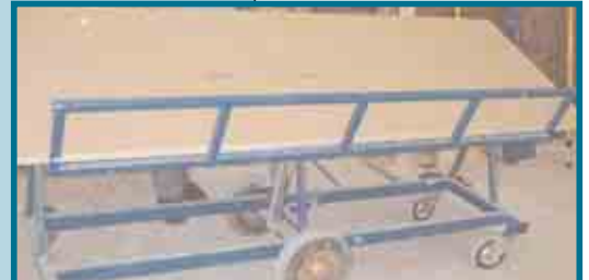
The bench allows boards to be wheeled from the pallet to the point of work without the need for them to be carried, reducing the risk of injury. Once in position, the trolley can be converted to a stable workbench that allows board preparation and subsequent handling to be completed at a suitable height, reducing the need to bend and stretch, and so reducing the risk of injury.
