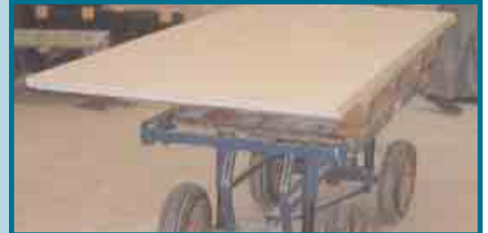
Using a lift truck on a larger site can prevent boards having to be manually handled to their point of use. Using the wheeled truck reduces the loading on the body and the associated risk of injury. This can increase productivity and reduce the manpower required to move a large quantity of boards. With this model, stacks of boards can be easily transferred to a set of purpose-made trestles, avoiding the need to handle each board.
