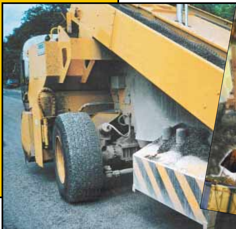
This chipper spreader reversed over a worker, who lost his leg in the accident
