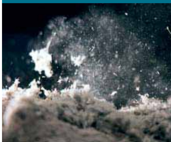
A piece of asbestos lagging being gently shaken
