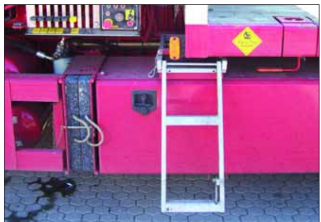
Figure 1 Fixed ladders providing safe and easy access
