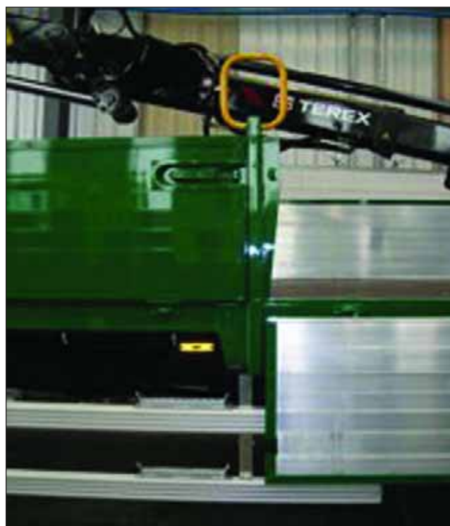
Figure 1 Side access steps and handhold.
