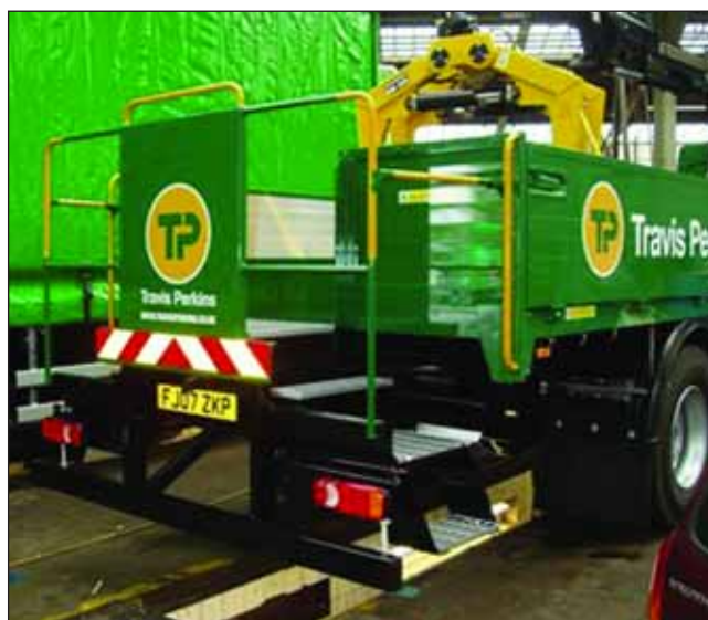
Figure 3 Bespoke rear access and working platform
