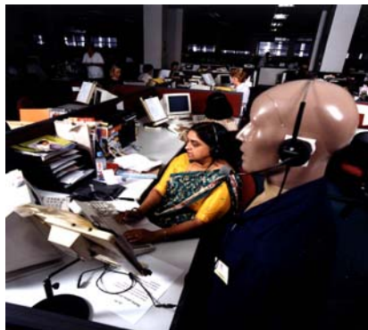
Use of head and torso simulator to assess noise exposure in call centres
