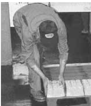
Production - unsafe repetitive bending, twisting and stretching
