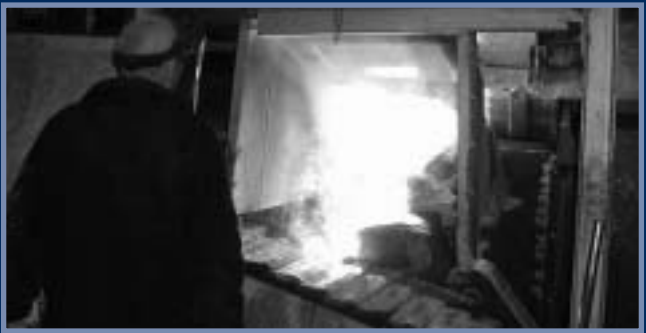
Figure 2 Induction furnace producing aluminium ingots
