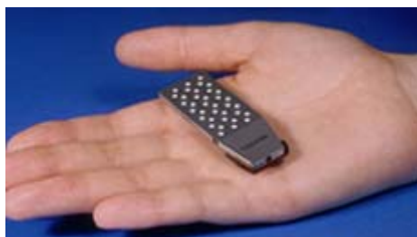
Figure 1 Small fuel cell prototype by Toshiba
