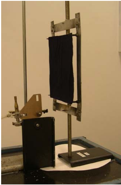
Figure 1 – Equipment set up with the burner in the standby position
